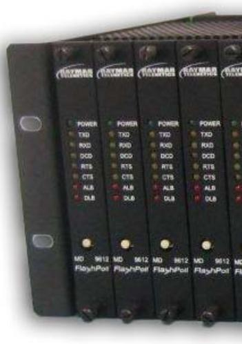
Figure 2-4. Modems Installed in the Rack
