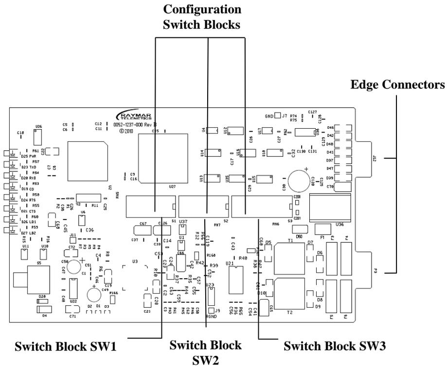
**Figure 2-2. Component View of Modem**
