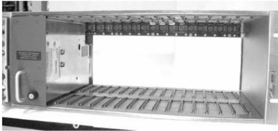
Figure 2-3. AC Power Module Installation
